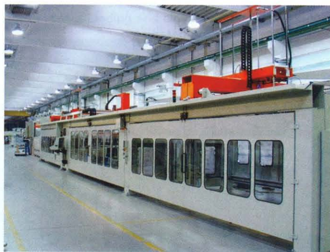
GEISS' highly innovative TT-in-one combines thermoforming and CNC trimming in a single unit
